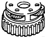
#9 REVERSE/OVERDRIVE RING GEAR THRUST BEARING ASSEMBLY 7F240
