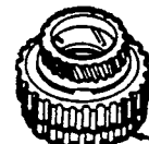
#5 LOW-INTERMEDIATE SUN GEAR THRUST BEARING ASSEMBLY 7H027
