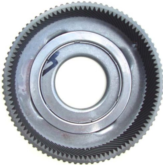
5R55W/S forward ring gear uses 101 teeth. The 5R55N has 85 teeth from 1999-01 and then in 2002 and later is the same as 5R55W/S models.
