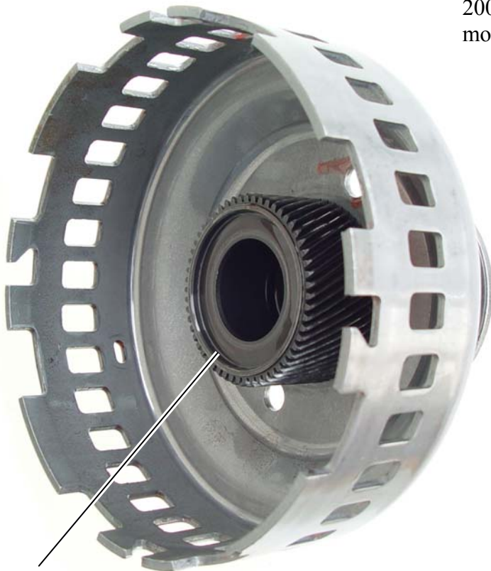
5R55W/S sun gear has 55 teeth and no roller bearing in bore. The 5R55N has 47 teeth with a roller bearing in the bore until 1999 and then is the same as the 5R55W/S
