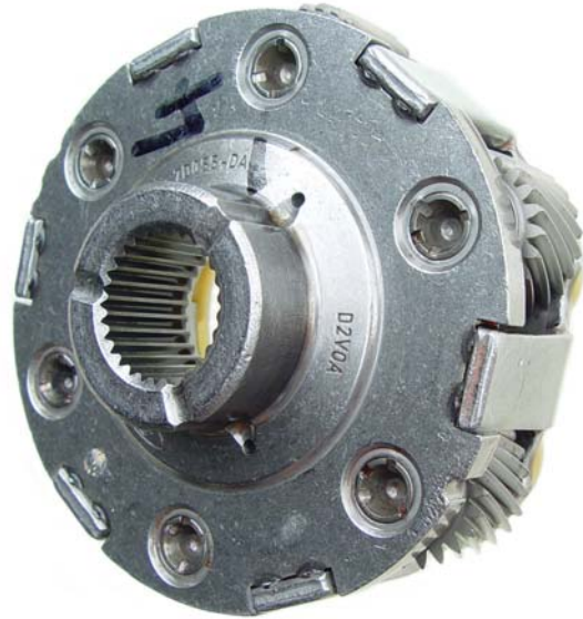
5R55W/S forward planetary is also different having 23 tooth pinion gears. The 5R55N uses 19 tooth gears until 2002 and then is the same as 5R55W/S models.
