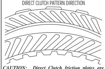
**CAUTION:** Direct Clutch friction plates are directional and must be installed with the internal tooth plate grooves facing clockwise, and the external tooth plates grooves facing counterclockwise, as shown above.
