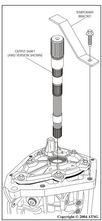
64. Remove and discard the 4WD adapter housing gasket, as shown in Figure 53.
